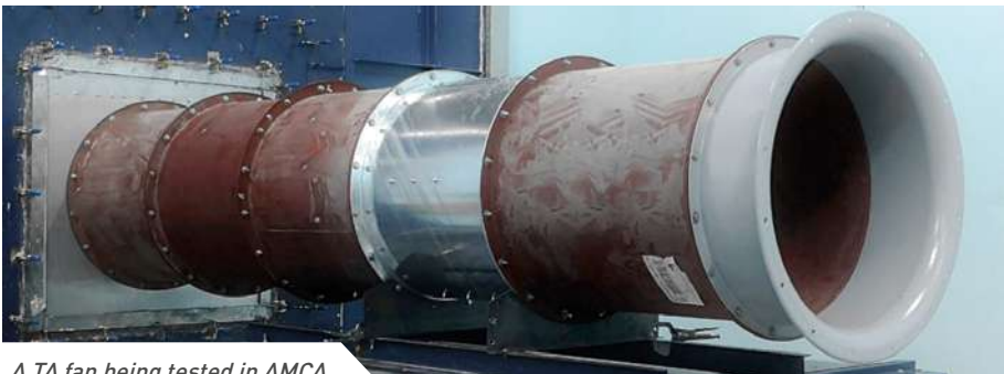
A TA fan being tested in AMCA
