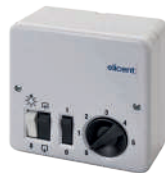
RVS/L 5 speed controller with on/off and light switch. Max load 0,5 A. IP42 protection. Size 118x118x58 mm.
