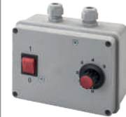
RVS PLUS EVO: 5 speed controller with on/off switch. Regulation up to 4 POLAR. Max load 1,5 A. IP 42 protection. Size 158x118x76 mm.
