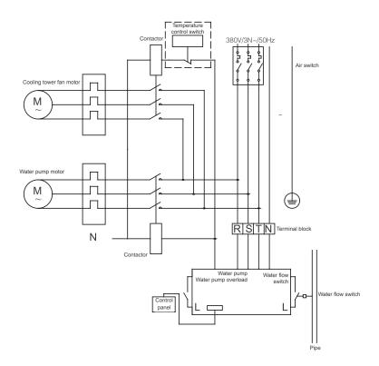
Note: If there is any requirement for refrigeration in winter, it is recommended to follow the wiring diagram.
